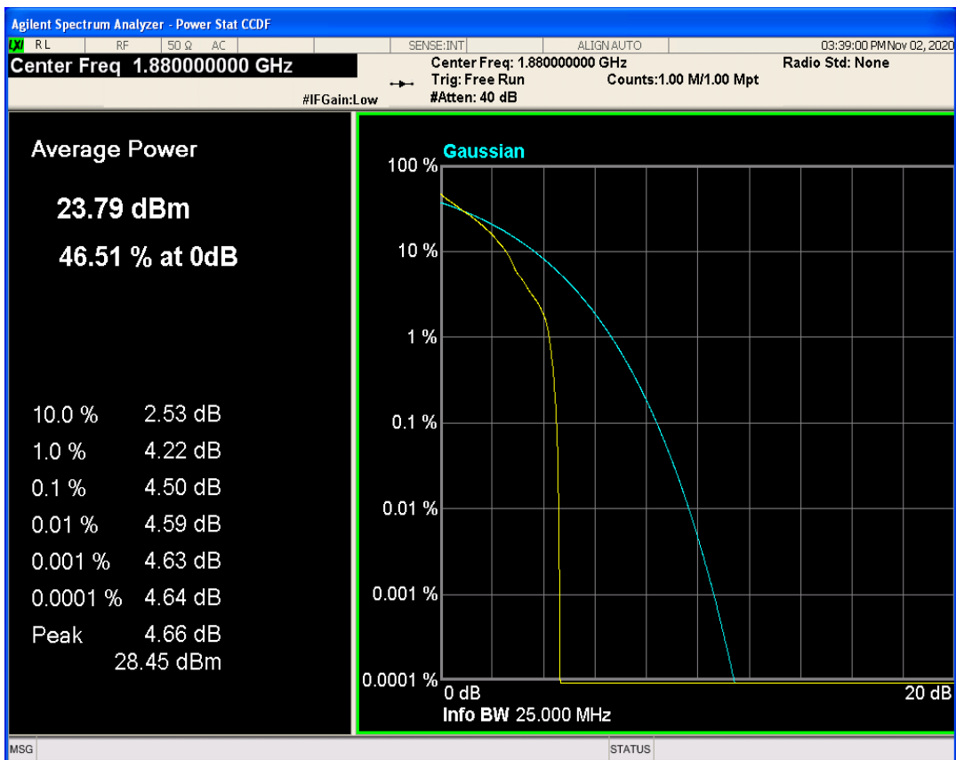
LTE Band2 QAM16 BW=20MHz Channel=18900 RB Size=1 Position=#0
