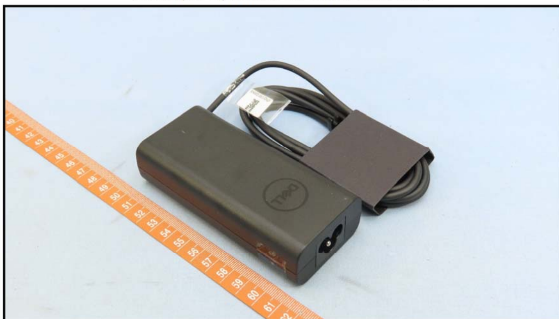
AC Adapter 6 (Brand: DELL, Model: LA65NM190)
