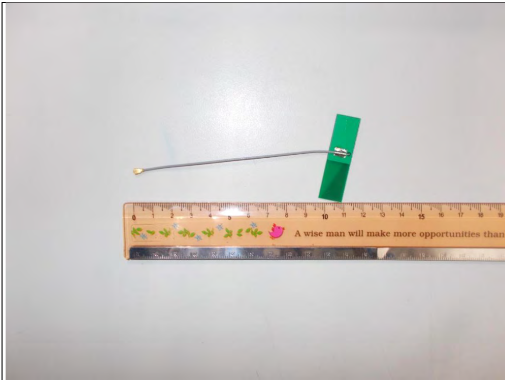
Antenna 7 (Brand: LAIRD ; Model: NanoBlue-IP04_MAF94045)
