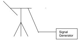
The spectrum analyzer is monitored to verify that the output of the signal generator produces a signal equal in amplitude to a previously measured spurious emission.
