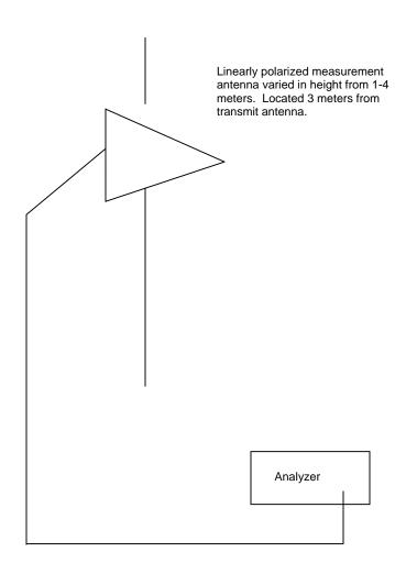
During field strength measurements, the amplitude and frequency of the highest emissions are noted. The transmitter is then replaced with a ½ wave dipole (at the same height) that is successively tuned to each of the highest spurious emissions. A signal generator is connected to the dipole (horn antenna for frequencies above 1 GHz), and its output is adjusted to match the level previously noted for each frequency.
