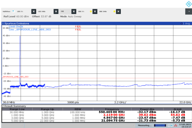
Figure 8.3-65: Conducted spurious emissions of multi-RAT operation, LTE 15 MHz + NR 5 MHz (bottom)
