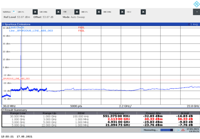
Figure 8.3-53: Conducted spurious emissions of WCDMA low channel, single-carrier operation
