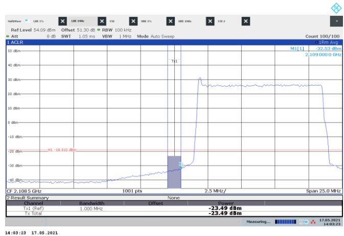
Figure 8.3-94: Conducted emission 1 MHz away from the lower band edge
