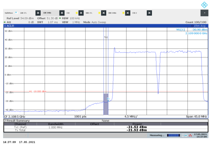
Figure 8.3-106: Conducted emission 1 MHz away from the lower band edge
