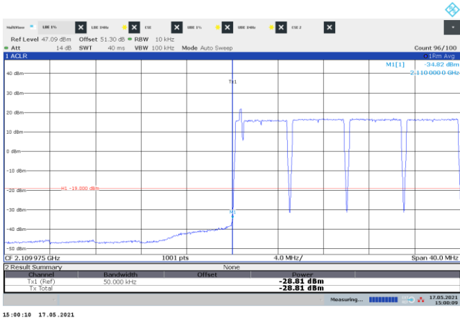
Figure 8.3-113: Conducted emission at the lower band edge
