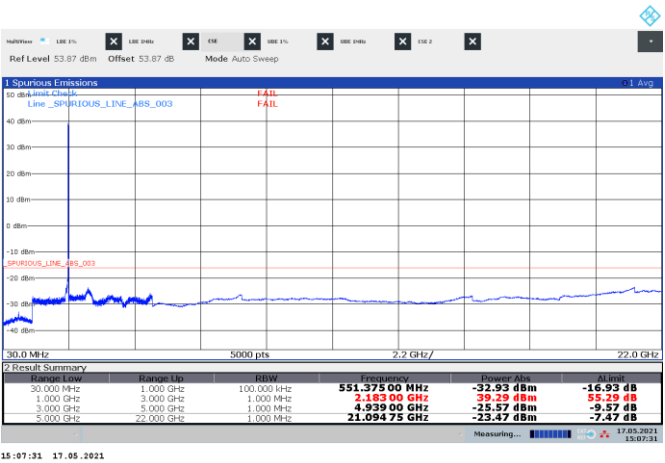
Figure 8.3-43: Conducted spurious emissions of NR 5 MHz four contiguous top channels, four-carrier operation
