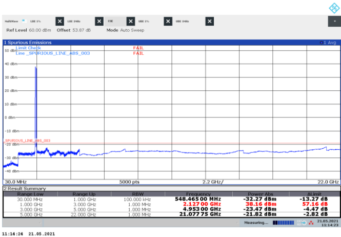
Figure 8.3-44: Conducted spurious emissions of NR 10 MHz two non-contiguous channels, two-carrier operation
