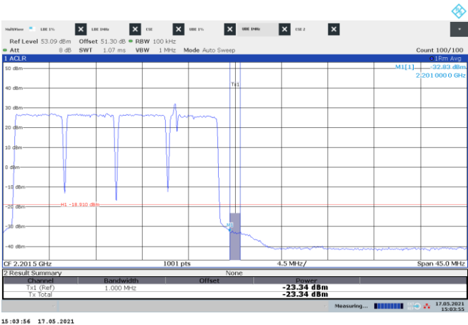
Figure 8.3-116: Conducted emission 1 MHz away from the upper band edge
