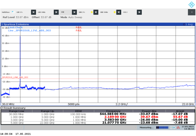
Figure 8.3-20: Conducted spurious emissions of LTE 10 MHz two contiguous top channels, two-carrier operation
