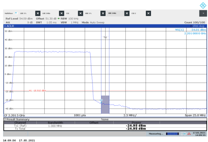
Figure 8.3-124: Conducted emission 1 MHz away from the upper band edge
