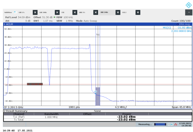
Figure 8.3-108: Conducted emission 1 MHz away from the upper band edge
