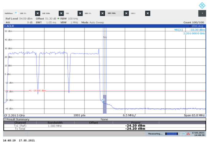
Figure 8.3-112: Conducted emission 1 MHz away from the upper band edge
