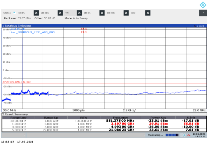
Figure 8.3-30: Conducted spurious emissions of NR 5 MHz top channel, single-carrier operation
