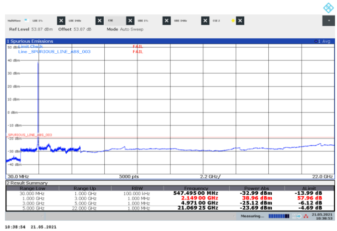
Figure 8.3-74: Conducted spurious emissions of multi-RAT operation, NR 10 MHz and LTE 5 MHz and WCDMA (mid)
