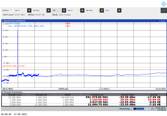
Figure 8.3-19: Conducted spurious emissions of LTE 10 MHz two contiguous mid channels, two-carrier operation
