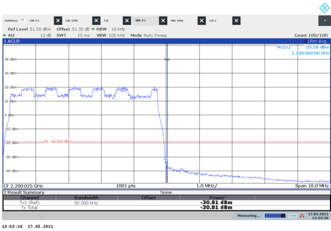
Figure 8.3-119: Conducted emission at the upper band edge
