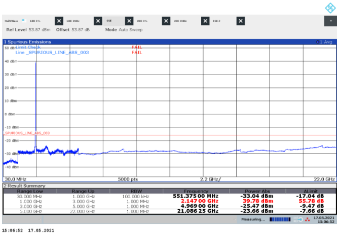
Figure 8.3-42: Conducted spurious emissions of NR 5 MHz four contiguous mid channels, four-carrier operation
