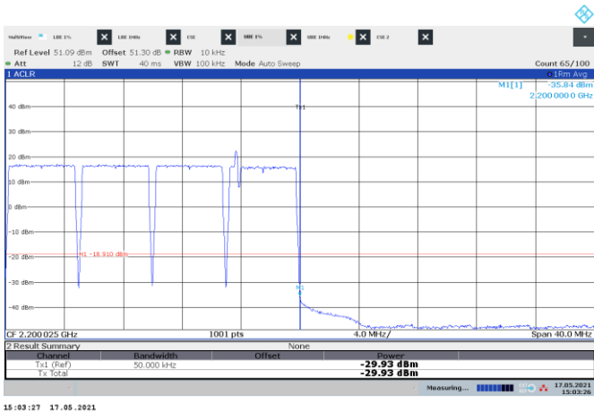
Figure 8.3-115: Conducted emission at the upper band edge
