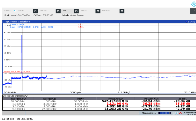
Figure 8.3-48: Conducted spurious emissions of NR 15 MHz two non-contiguous channels, two-carrier operation
