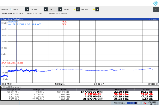
Figure 8.3-66: Conducted spurious emissions of multi-RAT operation, LTE 15 MHz + NR 5 MHz (mid)
