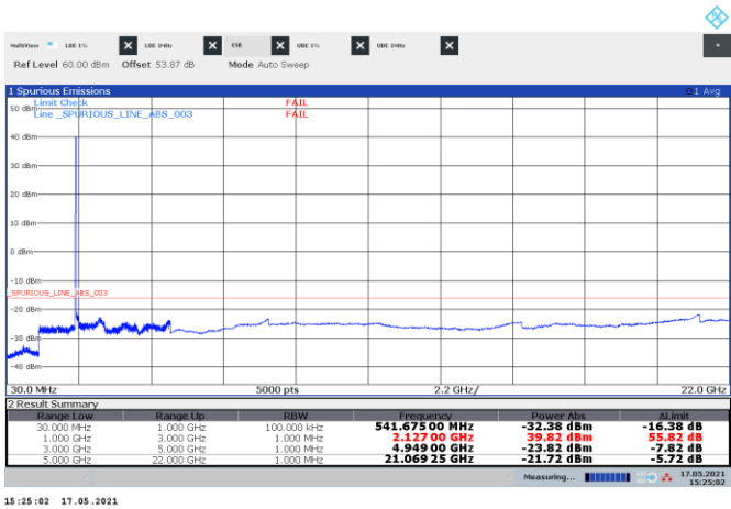
Figure 8.3-79: Conducted spurious emissions of multi-RAT operation, NR 15 MHz + WCDMA (bottom)
