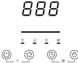
After the unit is powered on, it enters standby mode.
