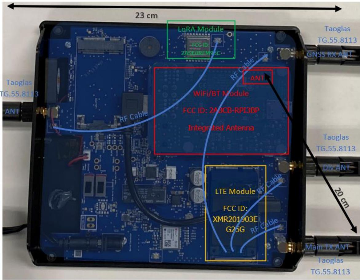
**DUT Description:** The GBP-2002 Gateway is used as part of the asset origination and full visibility Trackonomy infrastructure. It communicates wirelessly with nearby infrastructure devices like plugs and tagged movable assets. It has cellular connectivity to connect with the Internet to transmit information.
