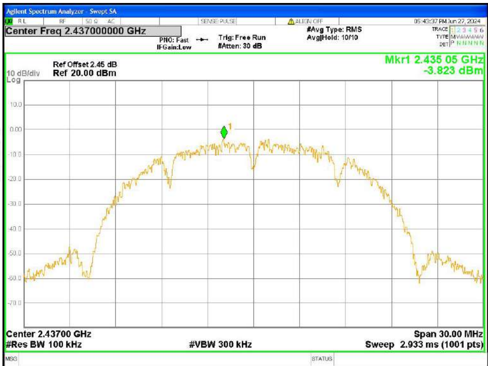
Tx. Spurious NVNT b 2437MHz Ant1 Ref
