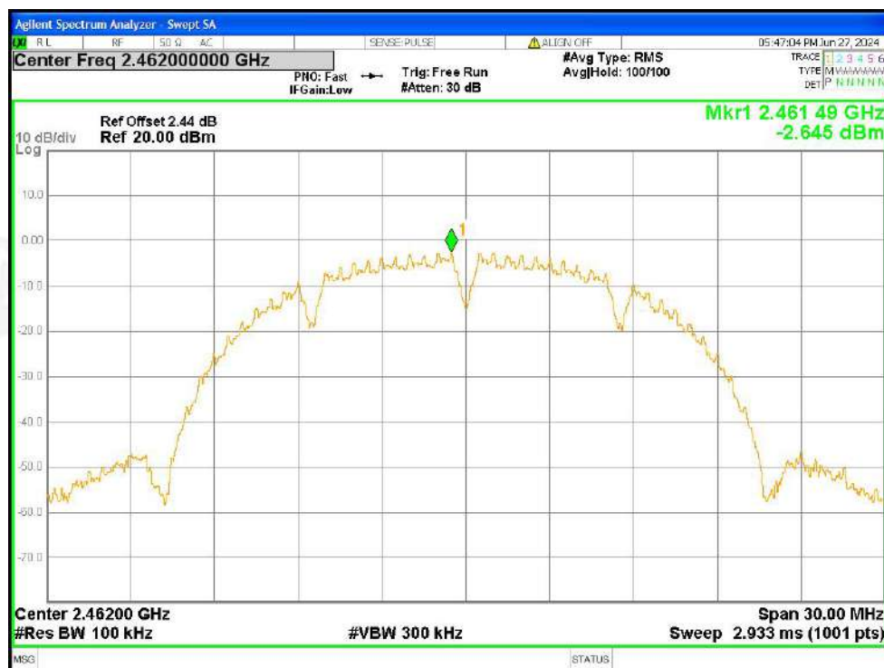
Tx. Spurious NVNT b 2462MHz Ant1 Ref
