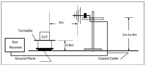
(c) For radiated emissions above 1000MHz
