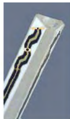
Figure 2.3 Probe Thick-Film Technique
