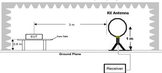
2. Radiated Emission Test Set-Up, Frequency below 1000MHz
