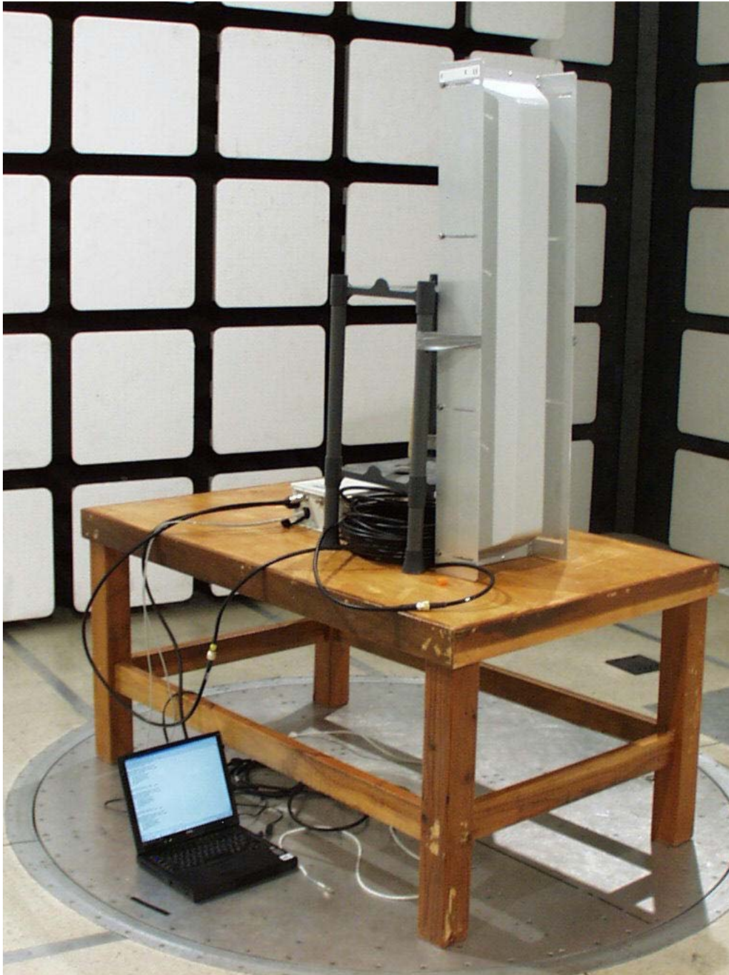
Radiated setup, base station configuration, sector antenna
