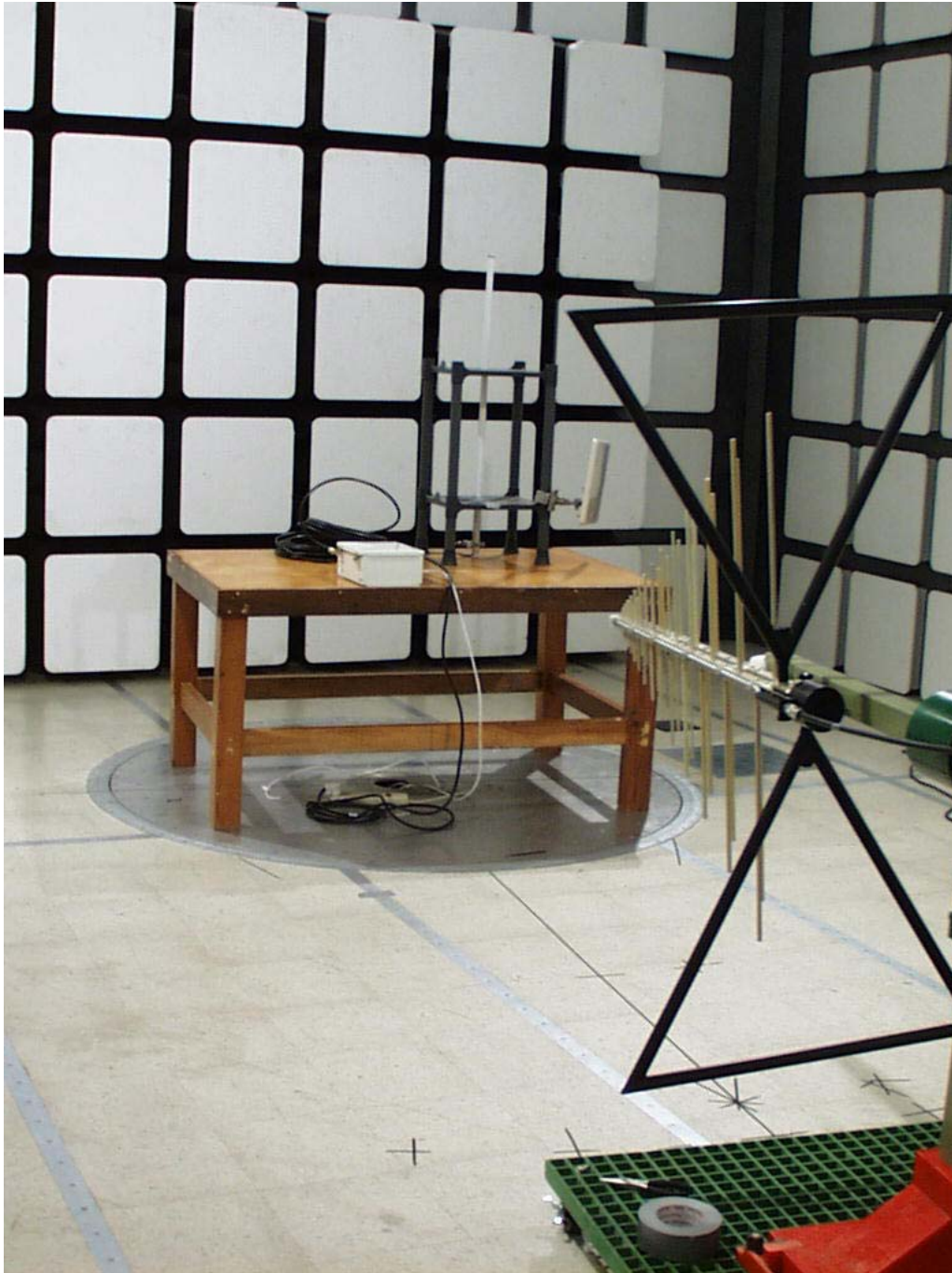
Radiated setup, base station configuration, omni antenna
