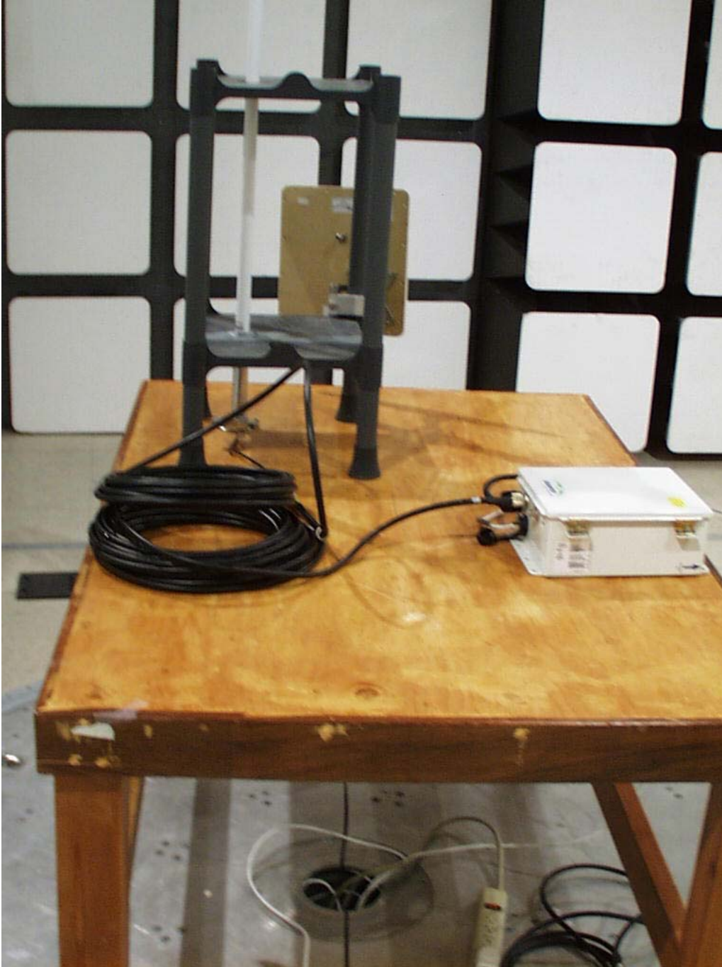
Base station configuration, radiated 30 – 1000 MHz
