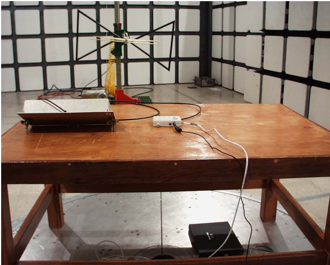
Subscriber unit, radiated emissions, 30 – 1000 MHz
