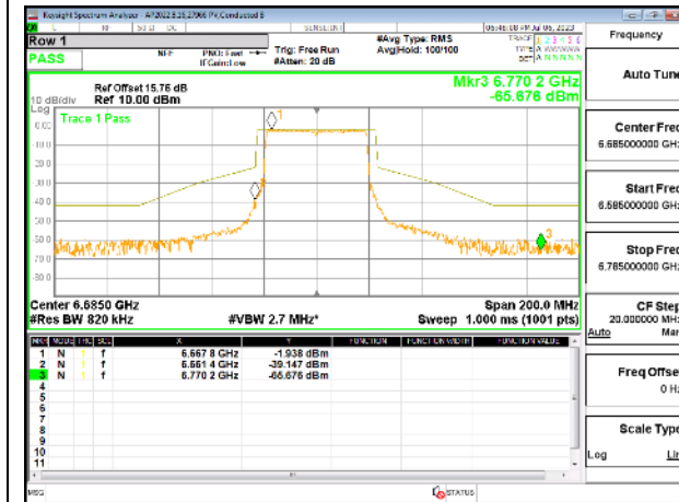
MID CHANNEL Antenna 3
