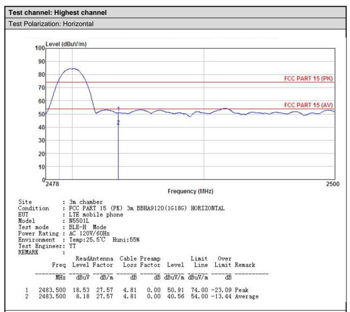
Final Level = Receiver Read level + Antenna Factor + Cable Loss - Preamplifier Factor.
