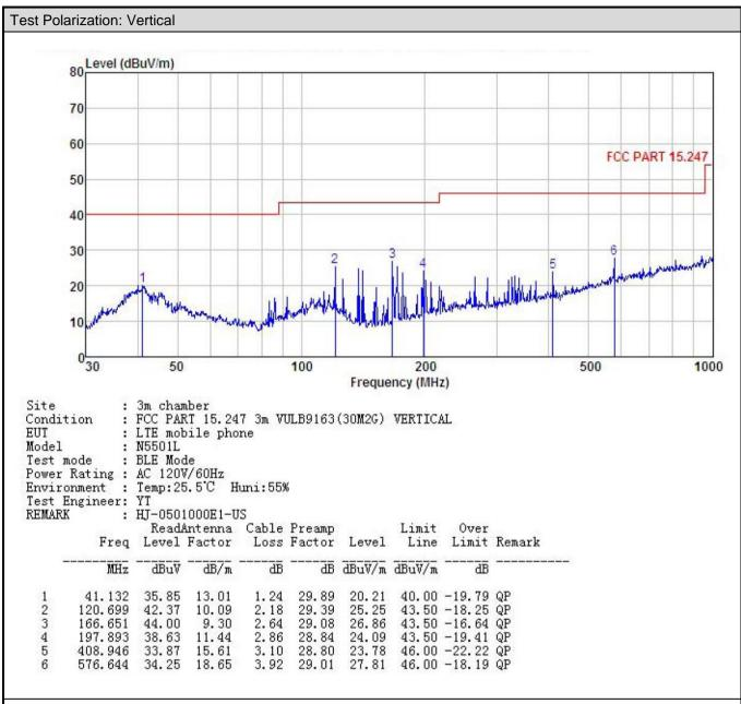
1. Final Level = Receiver Read level + Antenna Factor + Cable Loss - Preamplifier Factor.
