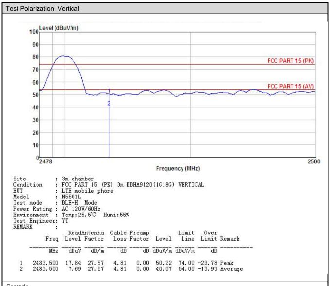
1. Final Level = Receiver Read level + Antenna Factor + Cable Loss - Preamplifier Factor.
