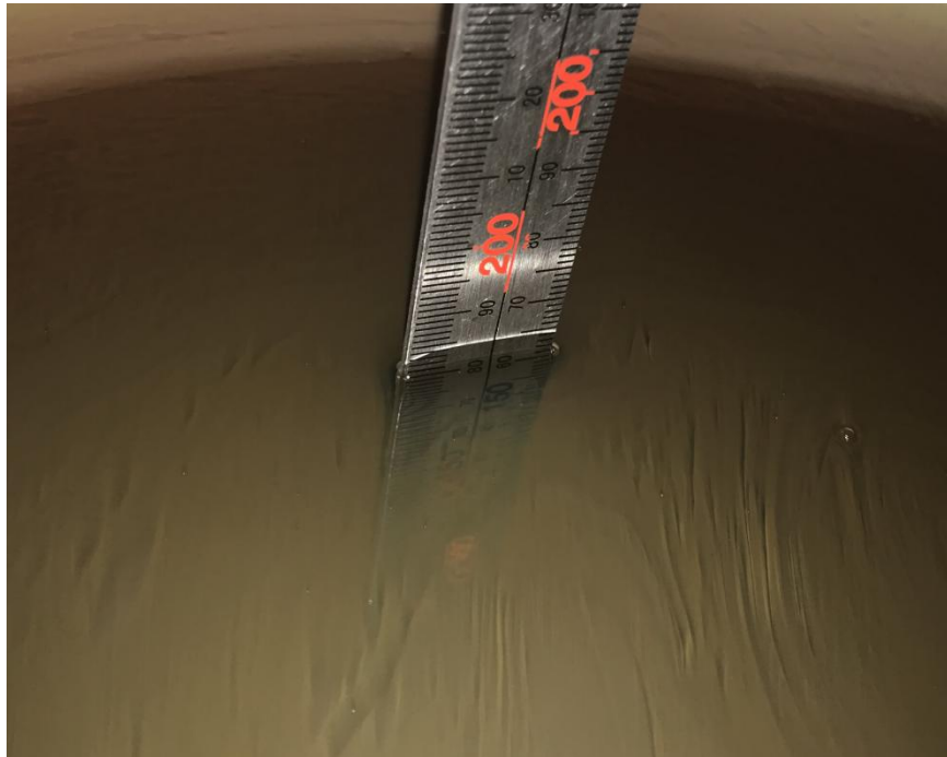
Liquid depth for SAR Measurement
