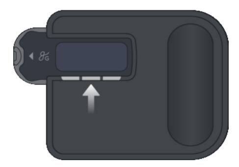
Lights off: Device is in standby mode; insert a test strip to wake the BGM and take a reading.
