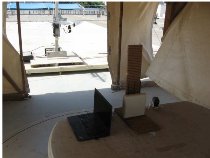
Figure 4. Radiated Emission Test, 200-1000MHz
