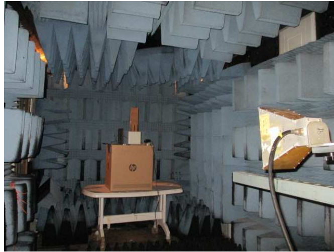
Figure 5. Radiated Emission Test, above 1000MHz
