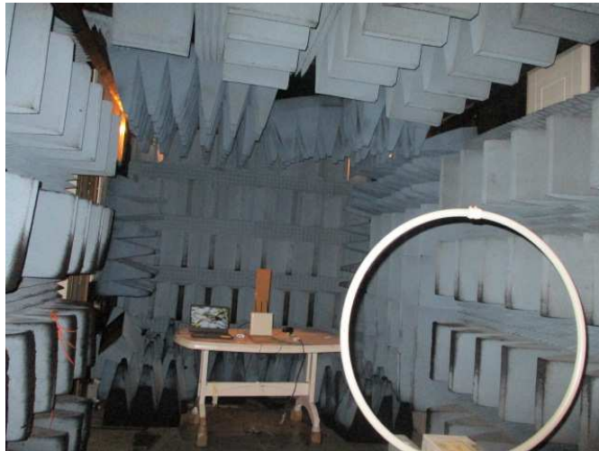
Figure 2. Radiated Emission Test, below 30MHz
