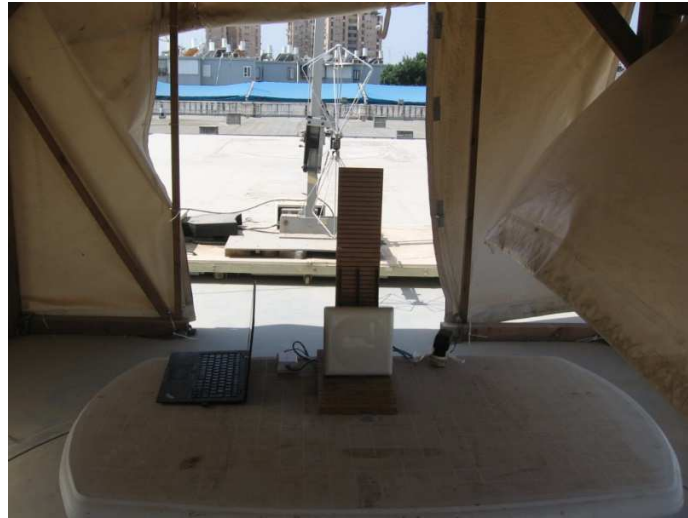
Figure 3. Radiated Emission Test, 30-200MHz
