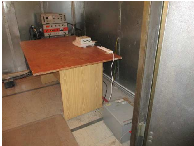
Figure 1. AC Line Conducted Emission Test
