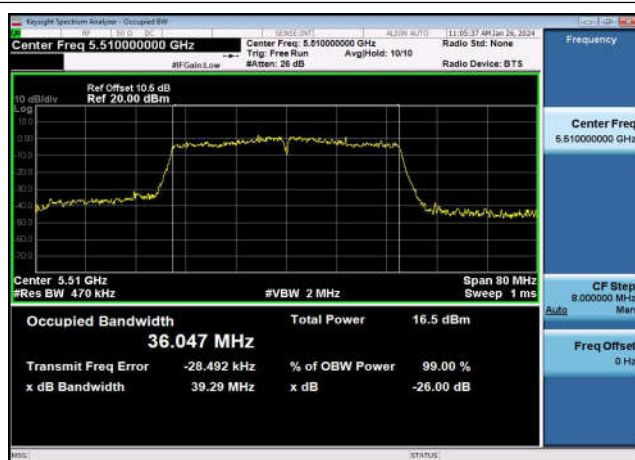
U-NII-2c 99% & 26dB Bandwidth-802.11ac(40MHz) ,5510MHz,Ant1
