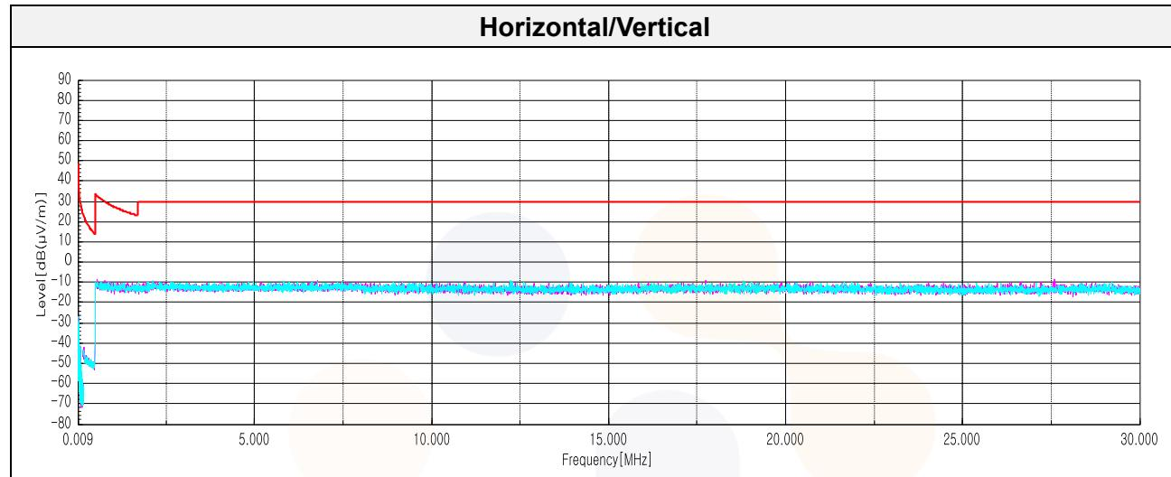
**Test results (Below 1 000 MHz) – Worst case: 802.11a / UNII 2A\_5 280 MHz**
