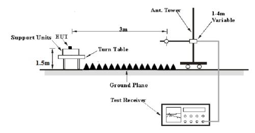
The radiated emission tests were performed in the 3 meters test site, using the setup accordance with the ANSI C63.10 - 2013. The specification used was the FCC § 15.209, 15.205 and 15.231.
