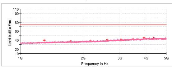
Corrected **Rx** Antenna Corrected Average Amplitude Turntable Frequency Margin Factor Limit Height Polar Degree (MHz) MaxPeak (**dB**) (dB/m) $(dB\mu V/m)$ (cm) (H/V)  $(dB\mu V/m)$ 39.24 200 V -10.6 1301.76 6 54.00 14.76 200 V 163 -8.6 60.83 20.80 1735.68 36.98 2169.60 38.09 200 Η 354 -7.0 60.83 19.51 2603.52 V 40.03 150 60 -5.3 60.83 18.40 3037.44 41.32 150 Η 2 -3.1 60.83 15.69 25 -1.9 3471.36 42.43 150 Η 60.83 16.72 Η 3905.28 45.14 200 335 0.0 54.00 8.86 V 4339.20 44.11 200 6 0.8 54.00 9.89
