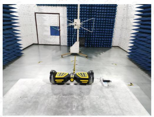
RADIATED EMISSION TEST SETUP ABOVE 1GHz
