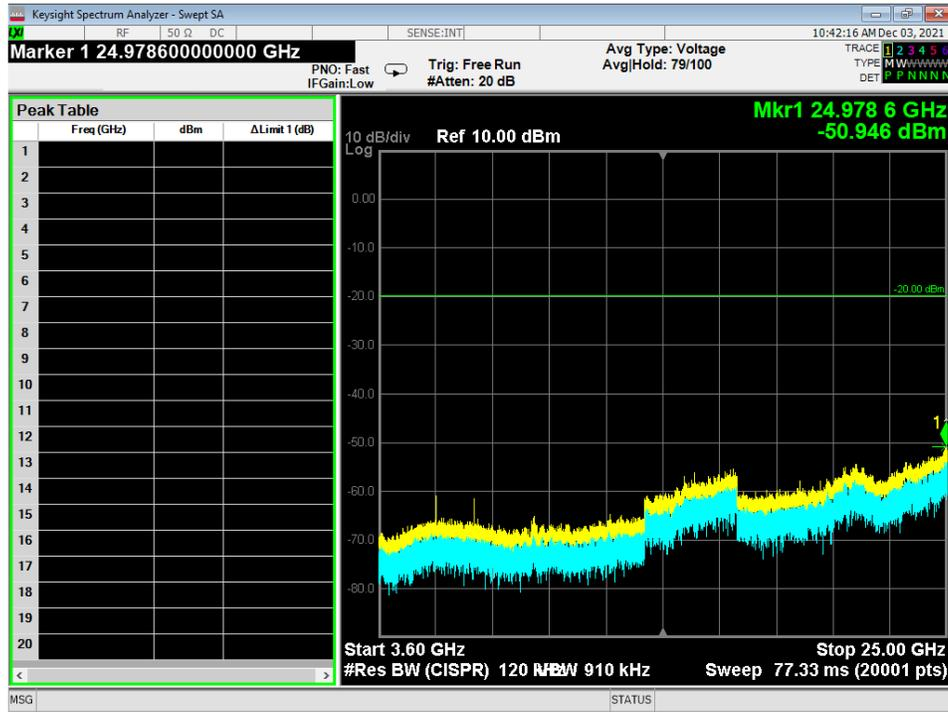
Figure 10 - Radiated Emissions Plot, 2EDR, 3.6G – 25G
