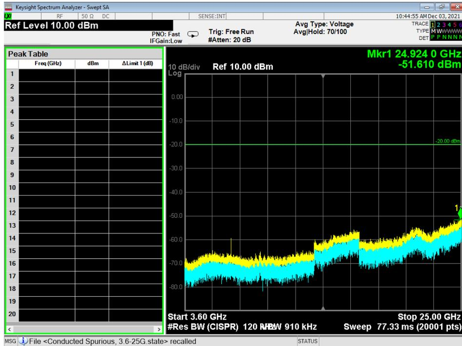
Figure 13 - Radiated Emissions Plot, 3EDR, 3.6G – 25G
