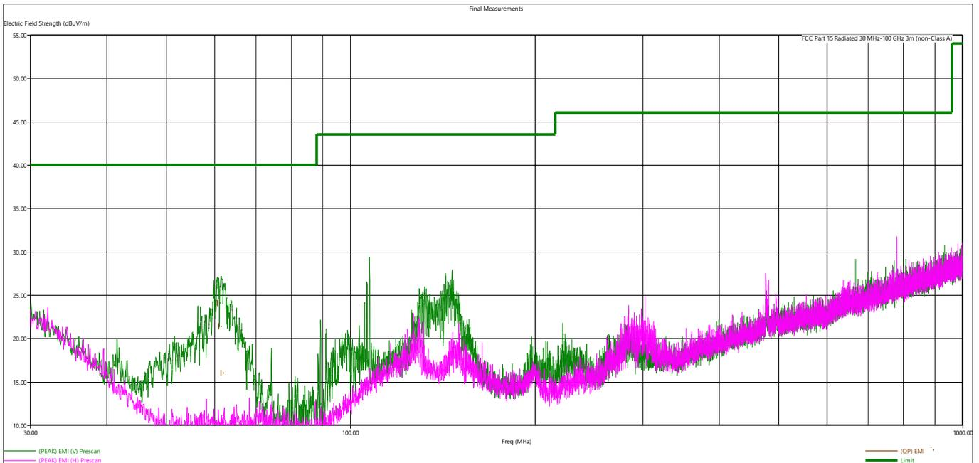
**Figure 6 - Radiated Emissions Plot, BT EDR 2MB**
