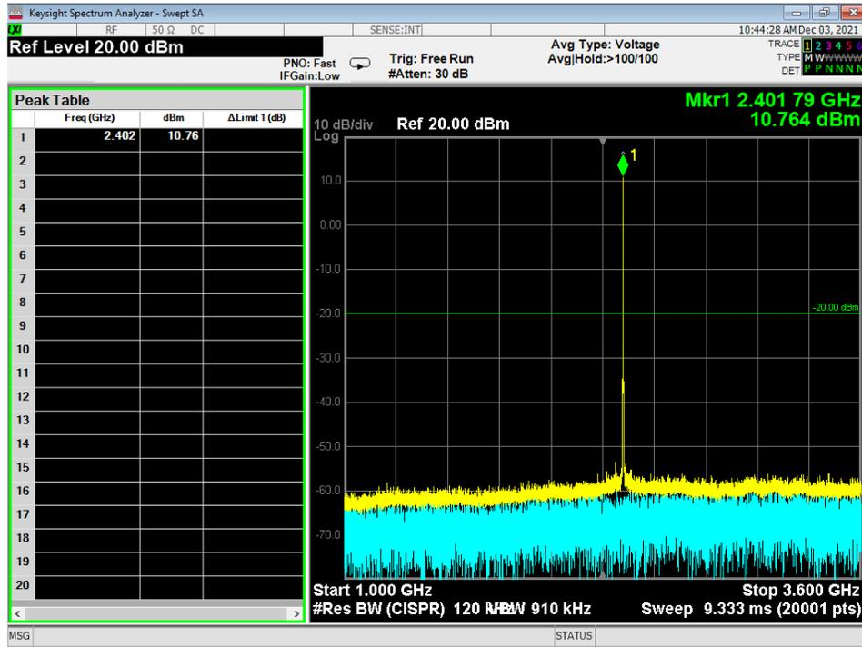
Figure 12 - Radiated Emissions Plot, 3EDR, 1G – 3.6G
