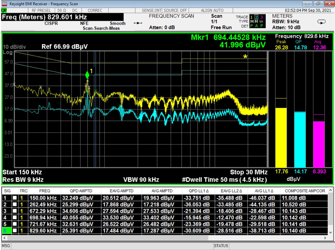
Figure 17 - Conducted Emissions Plot, Neutral, IDLE
