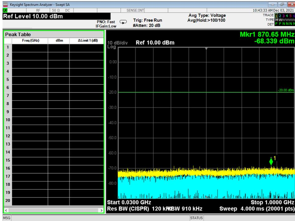
Figure 11 - Radiated Emissions Plot, 3EDR, 30M – 1G
