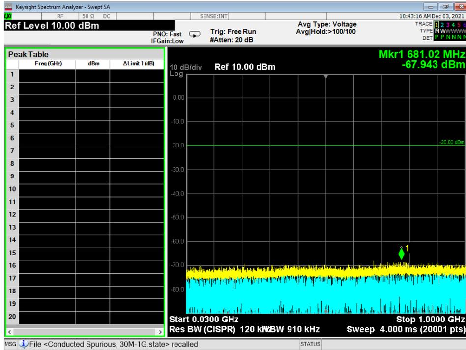
Figure 8 - Radiated Emissions Plot, 2EDR, 30M – 1G
