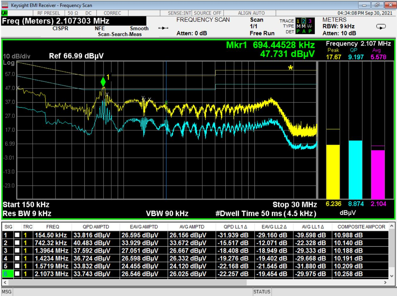
Figure 14 - Conducted Emissions Plot, Line, TX
