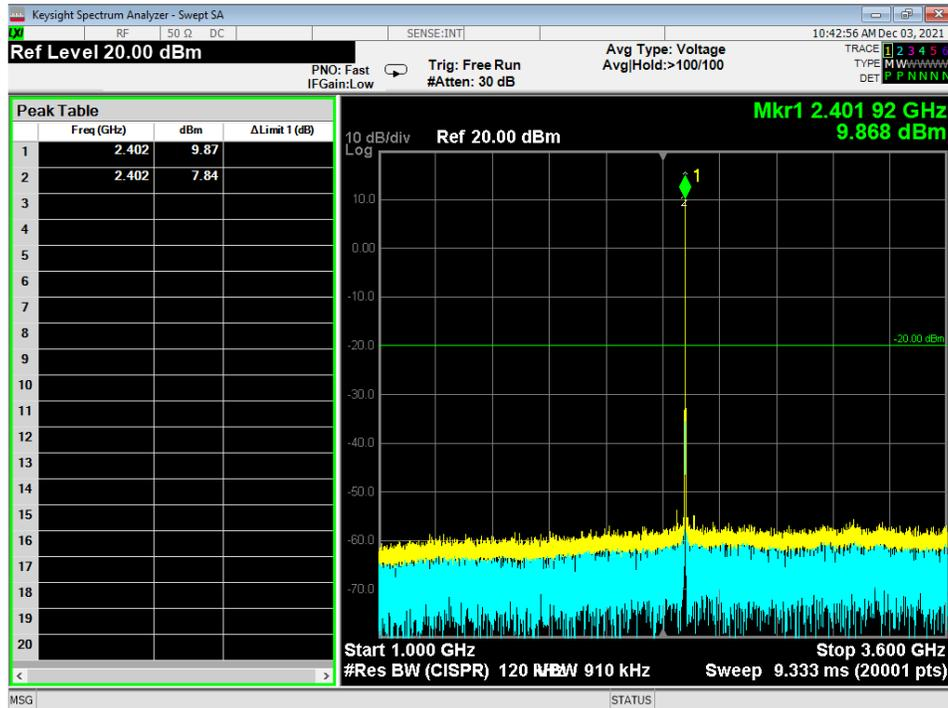
Figure 9 - Radiated Emissions Plot, 2EDR, 1G – 3.6G
