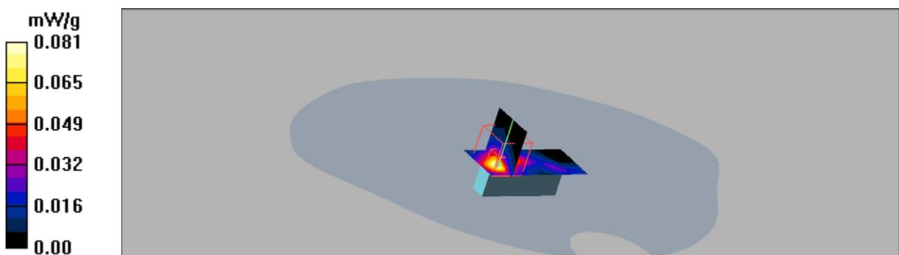
**Camera left-5.8 GHz a mode High Channel****DUT: Camera top; Type: Body worn pov camera;**
