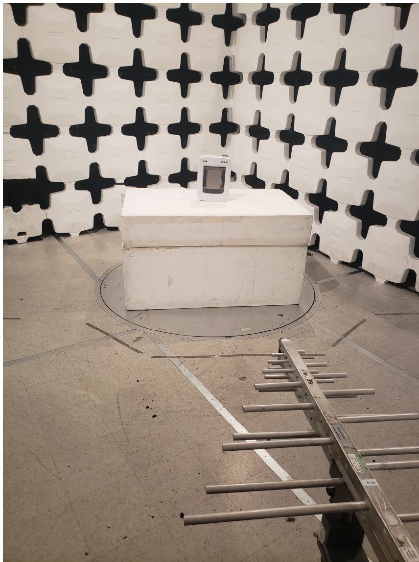
Figure 4. Radiated Emissions Test Setup, 200 MHz to 1 GHz
