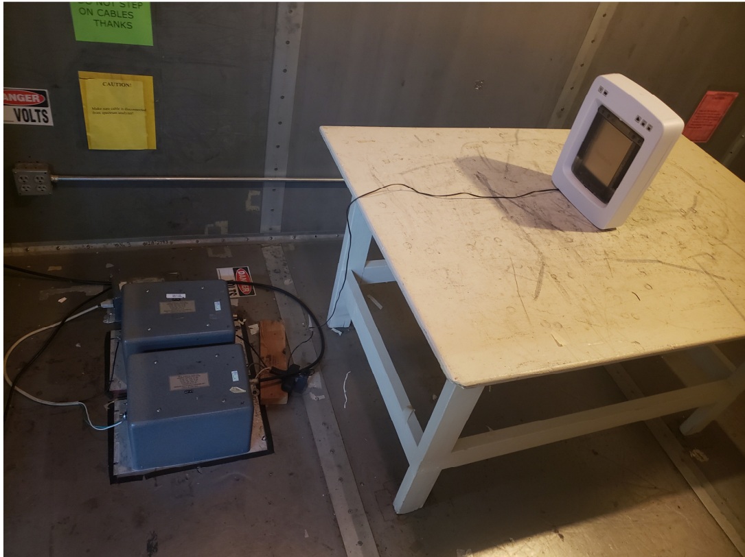
Figure 6. Powerline Conducted Emission Test Setup
