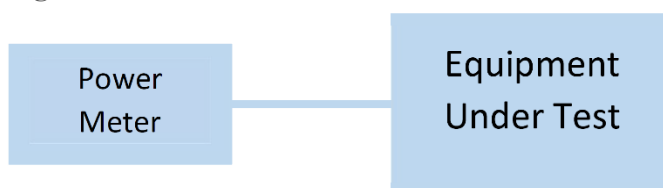
Figure 3: Output Power Measurement
