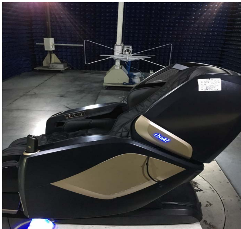
Photograph of set-up for Radiated Emission below 1GHz
