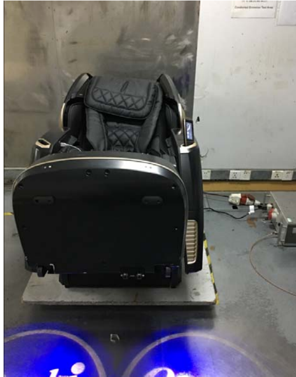
Photograph of set-up for AC Power line Conducted Emission
