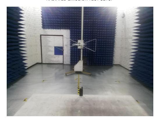
RADIATED EMISSION ABOVE 1G TEST SETUP
