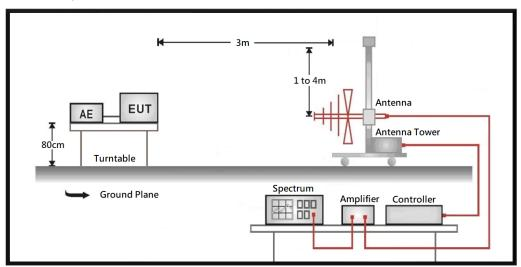
Radiated Spurious Measurement: above 1GHz
