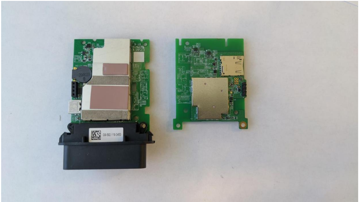
Mainboard with shielding removed
