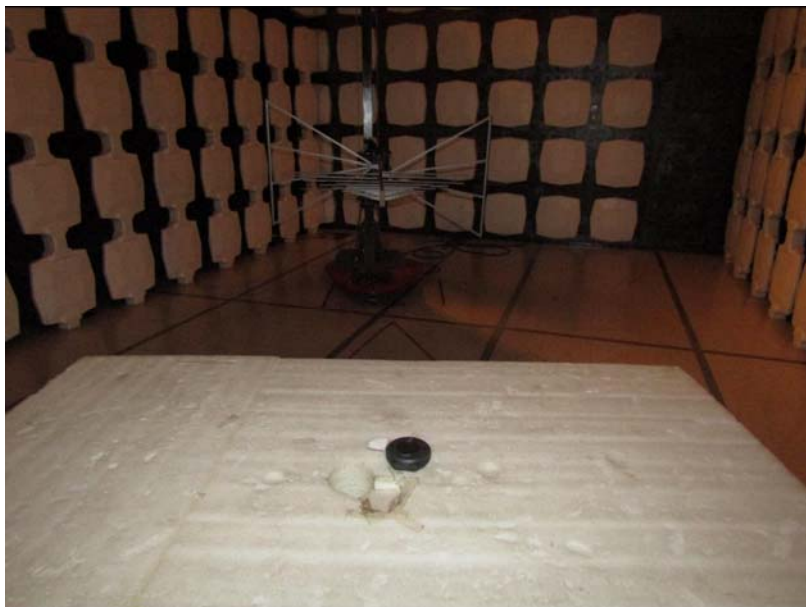
Measurement of Radiated Emission Test Set Up
