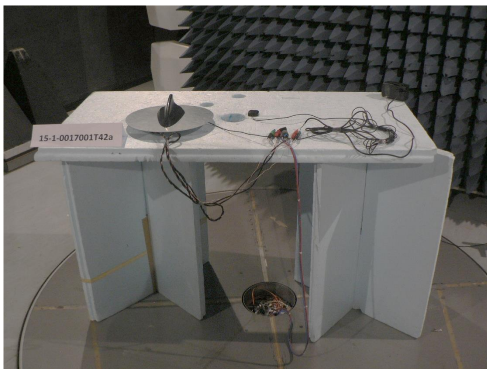
Photograph 3: Radiated measurements in semi-anechoic room (close view)
