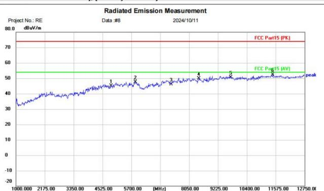
Site Polarization: Vertical Temperature: (C)
