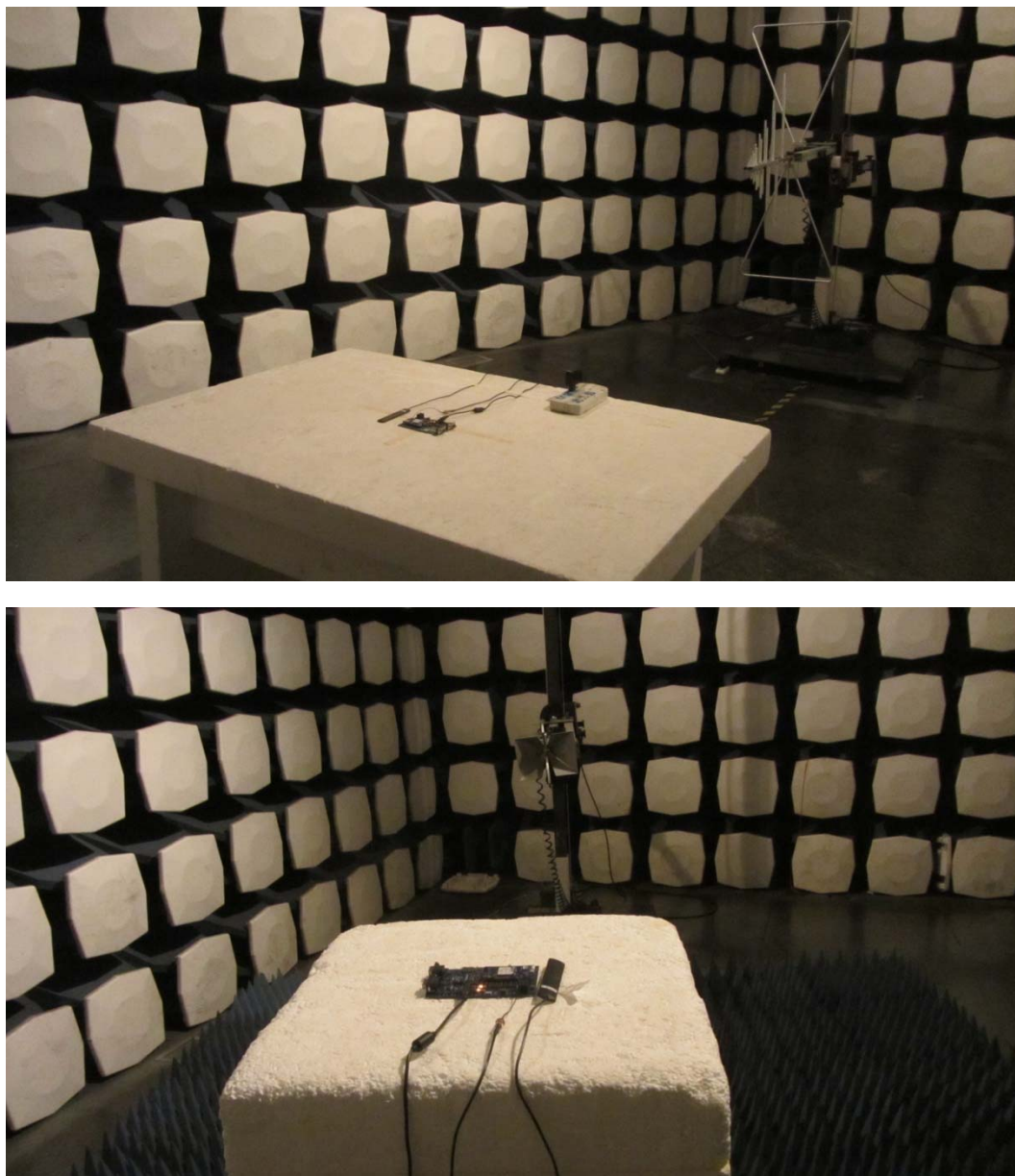
Picture 2: Radiated Spurious Emissions Test setup
