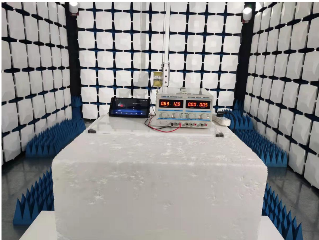
Above 1GHz for radiated emission test setup
