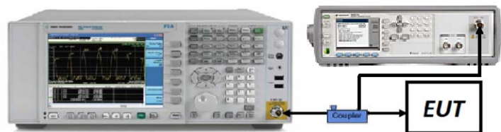
Figure 7-6. Test Instrument & Measurement Setup
