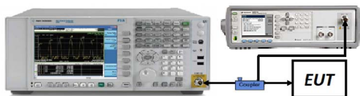
Figure 7-5. Test Instrument & Measurement Setup
