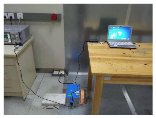
RADIATE EMISSION TEST SETUP ABOVE 1GHz
