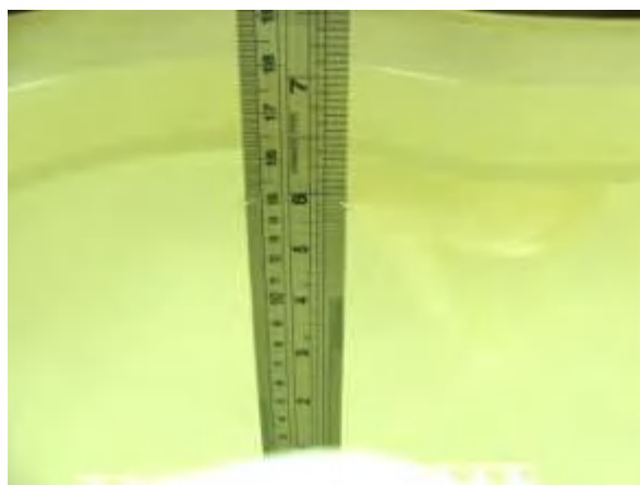
Photo of Liquid Height for Head SAR
