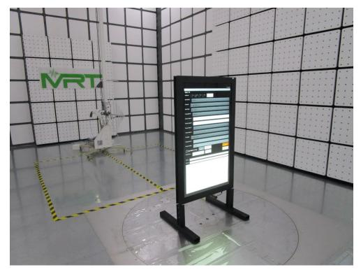
Test Mode 1 ~ Mode4 Description: Radiated Emission Test Setup for above 1GHz
