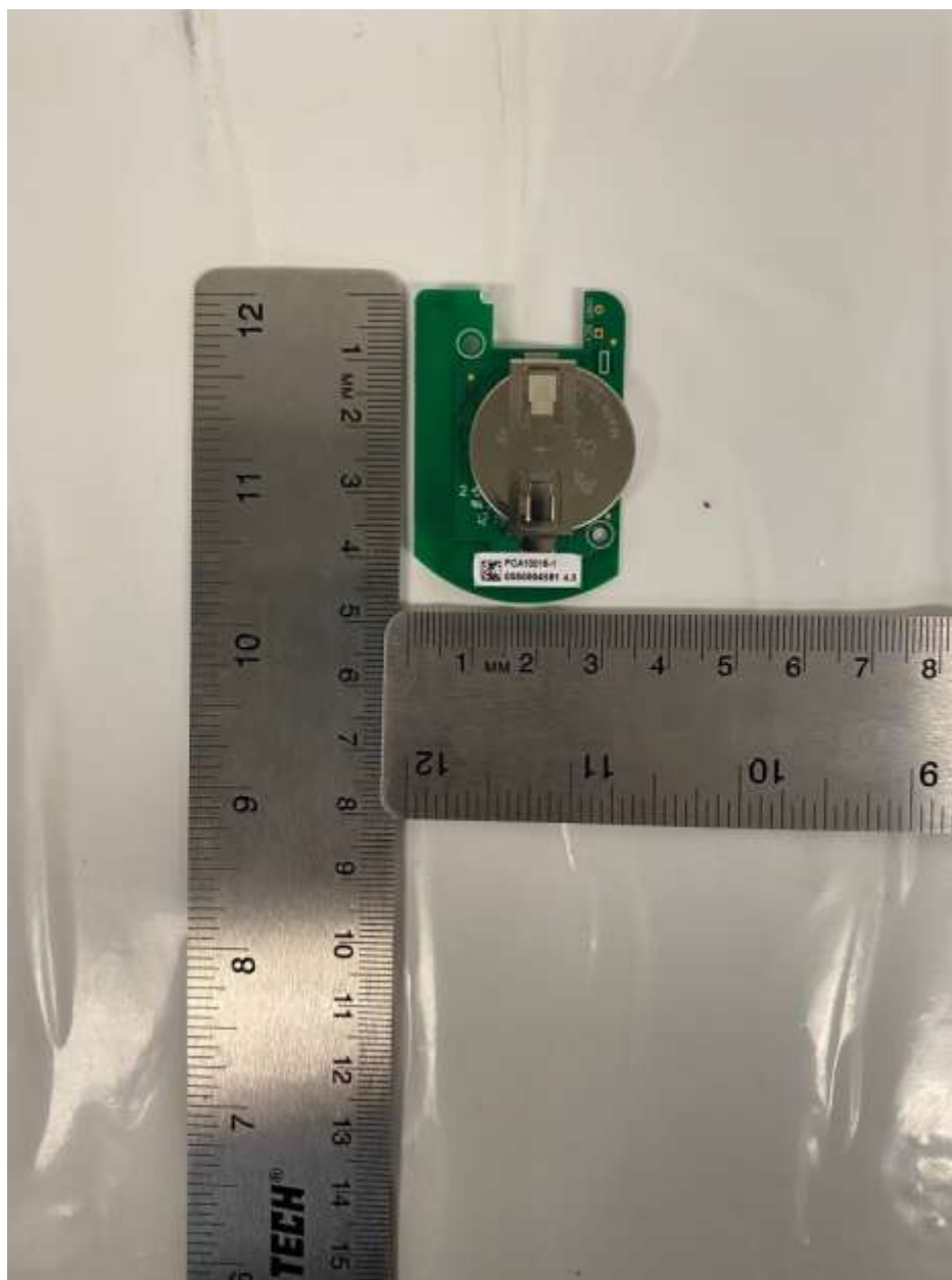
Figure 3. PCB Side 2 (with Battery)
