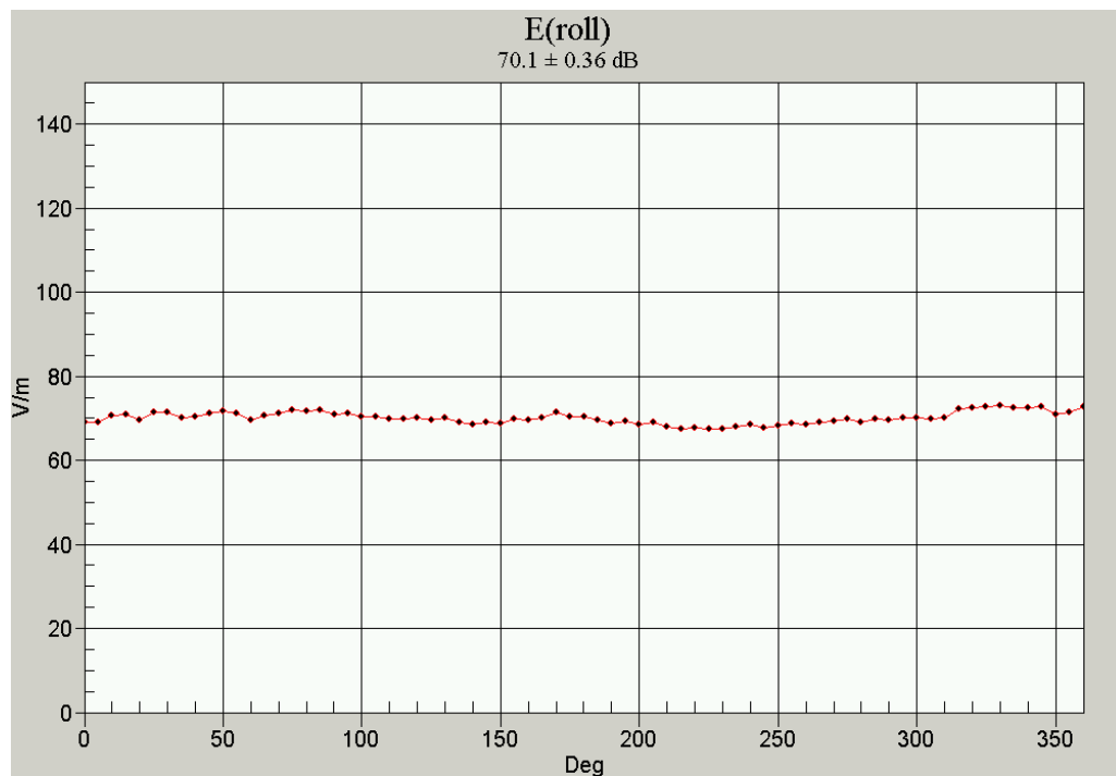
Figure 29 Worst-Case Probe Rotation about Azimuth axis
