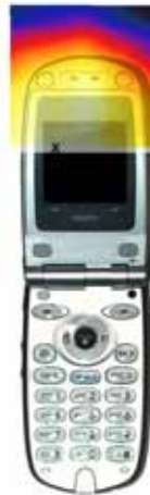
Figure 27 Sample E-field Scan Overlay
