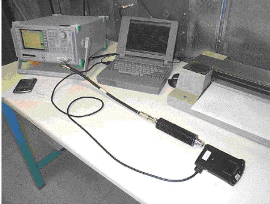
Testing Spurious Radiation from Transmitter at Antenna Port on DWV 100D Wireless Modem connected to PC only
