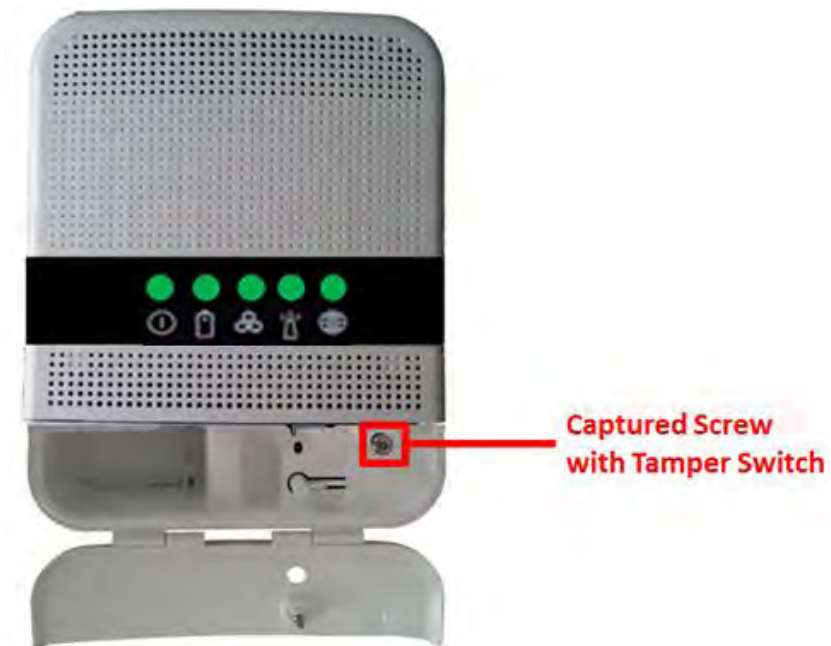
Figure 4: Mounting Plate Captured Screw with Tamper Switch
