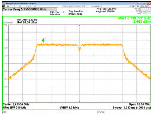
(802.11ac40) PSD plot on channel 159
