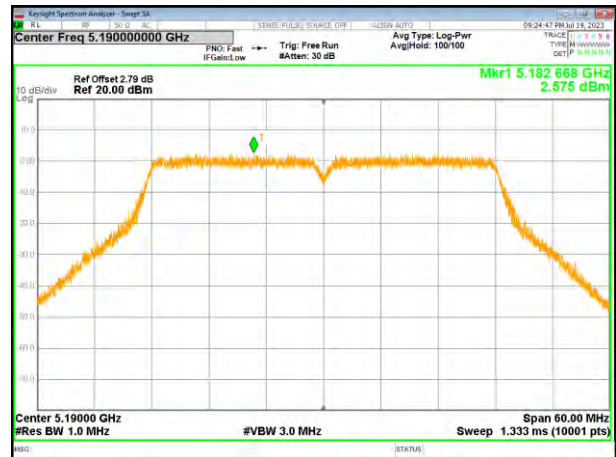
(802.11n40) PSD plot on channel 46
