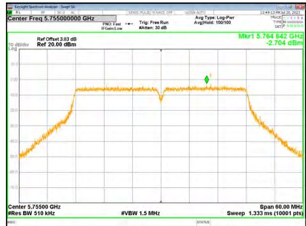
(802.11n40) PSD plot on channel 159
