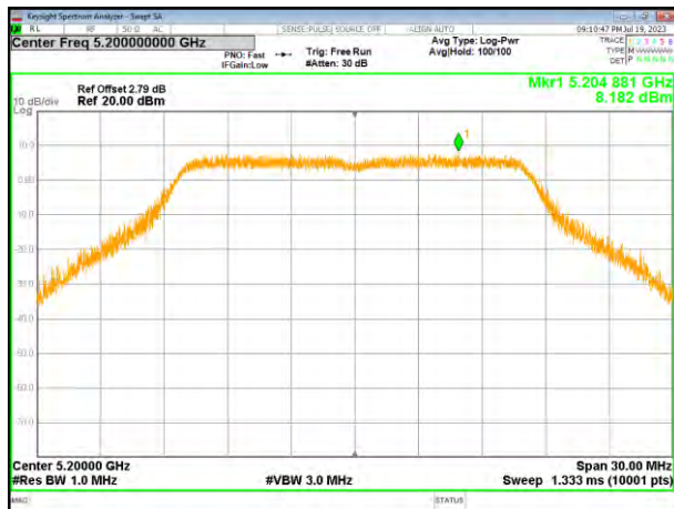
(802.11a) PSD plot on channel 40
