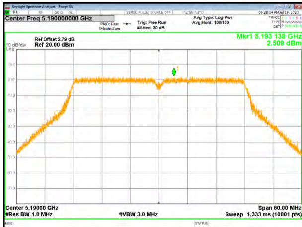
(802.11ac40) PSD plot on channel 46
