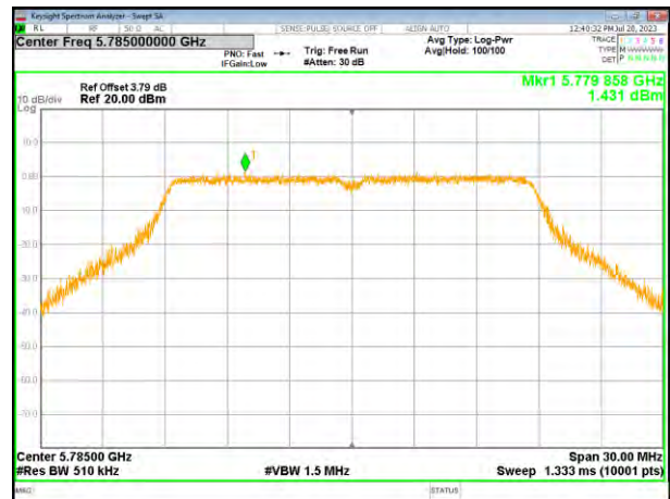
(802.11n20) PSD plot on channel 157
