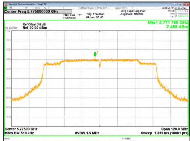
(802.11ac80) PSD plot on channel 155
