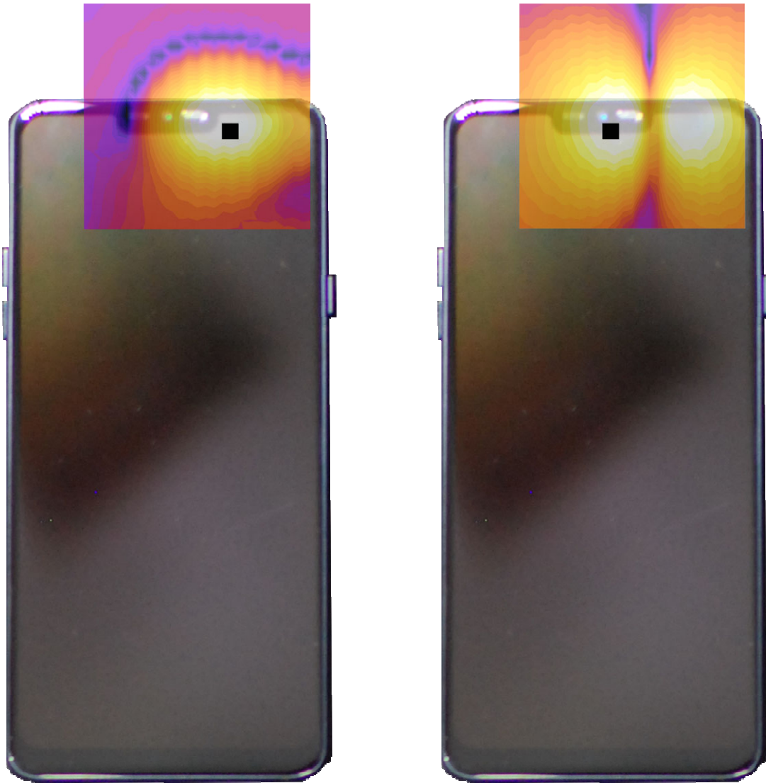
Figure 16-3 T-Coil Scan Overlay Magnetic Field Distributions
