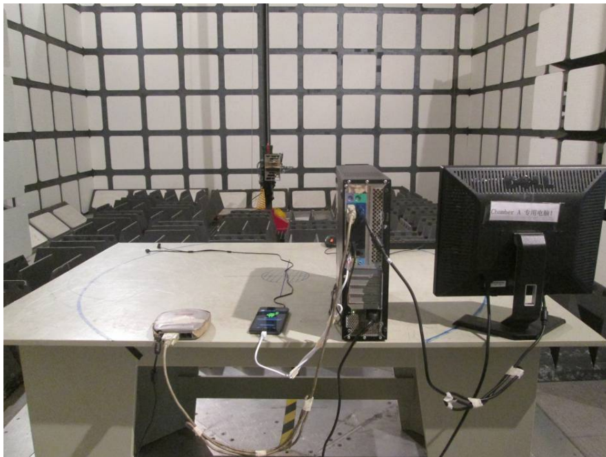
Radiated Emissions – Rear View (Above 1 GHz)
