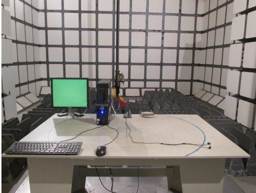
Radiated Emissions – Front View (Above 1 GHz)
