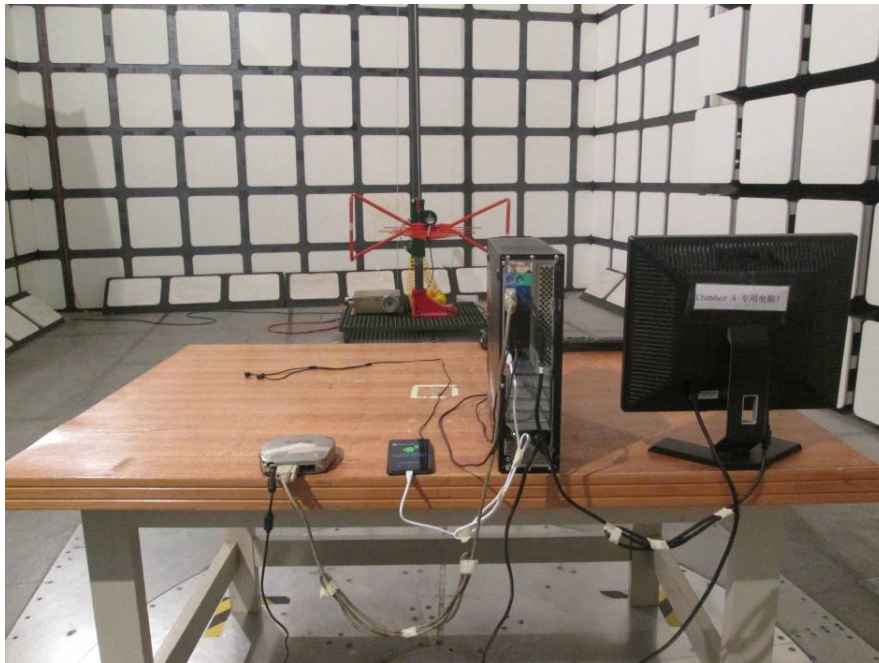
Radiated Emissions – Rear View (Below 1 GHz)
