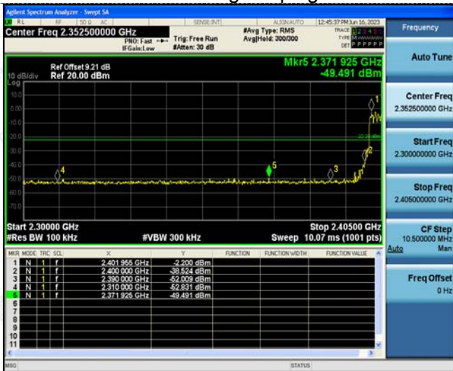
Left Band edge hopping on
