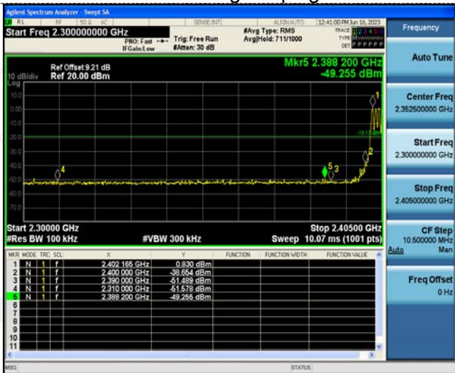
Left Band edge hopping on
