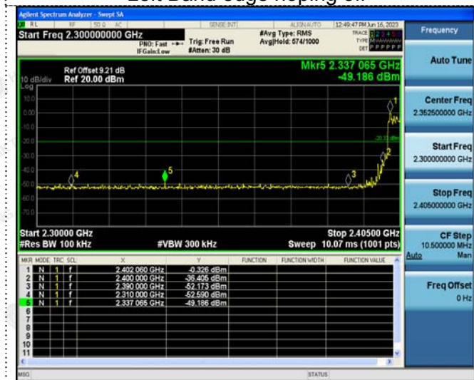
Left Band edge hopping on
