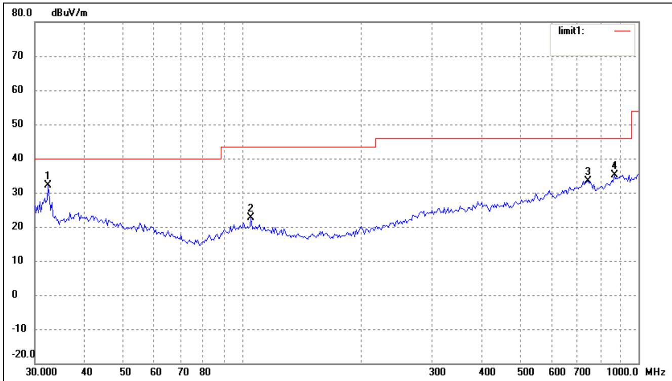
*Operating Condition:* 802.11n-HT20 Transmitting High Channel-2462MHz
