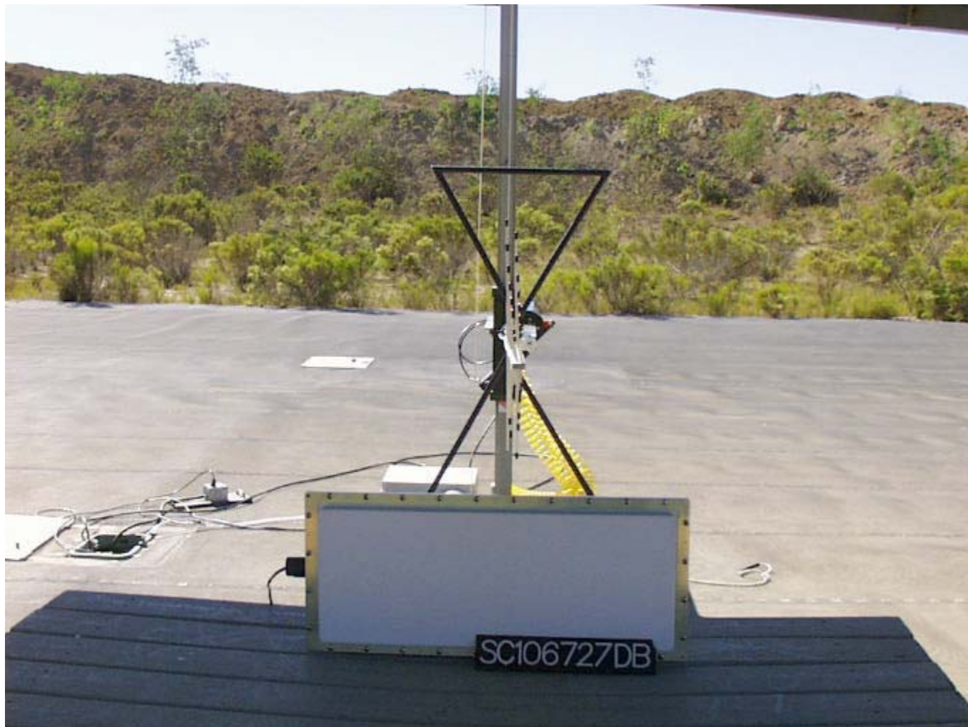
Photograph of Test Setup: Radiated Emissions
