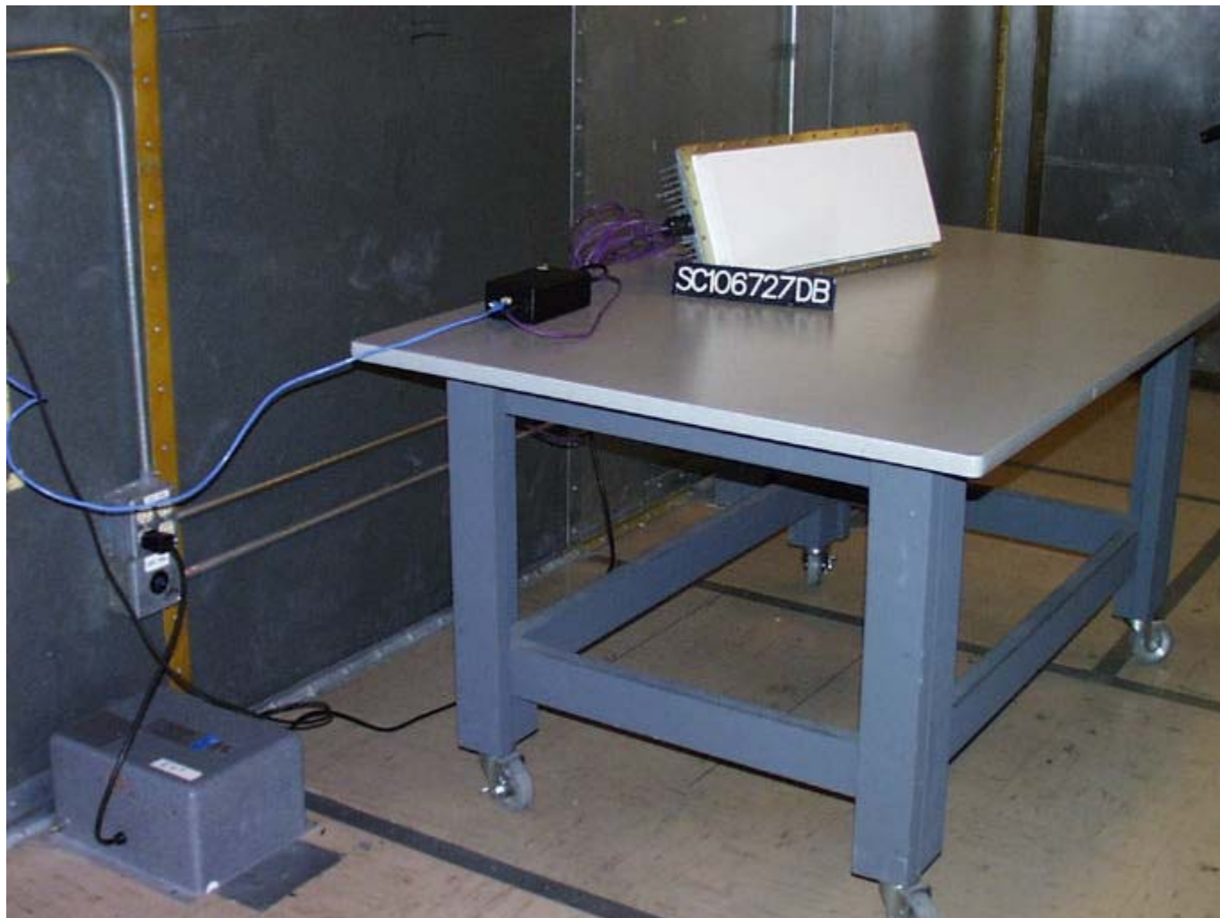
Photograph of Test Setup: Conducted Emission
