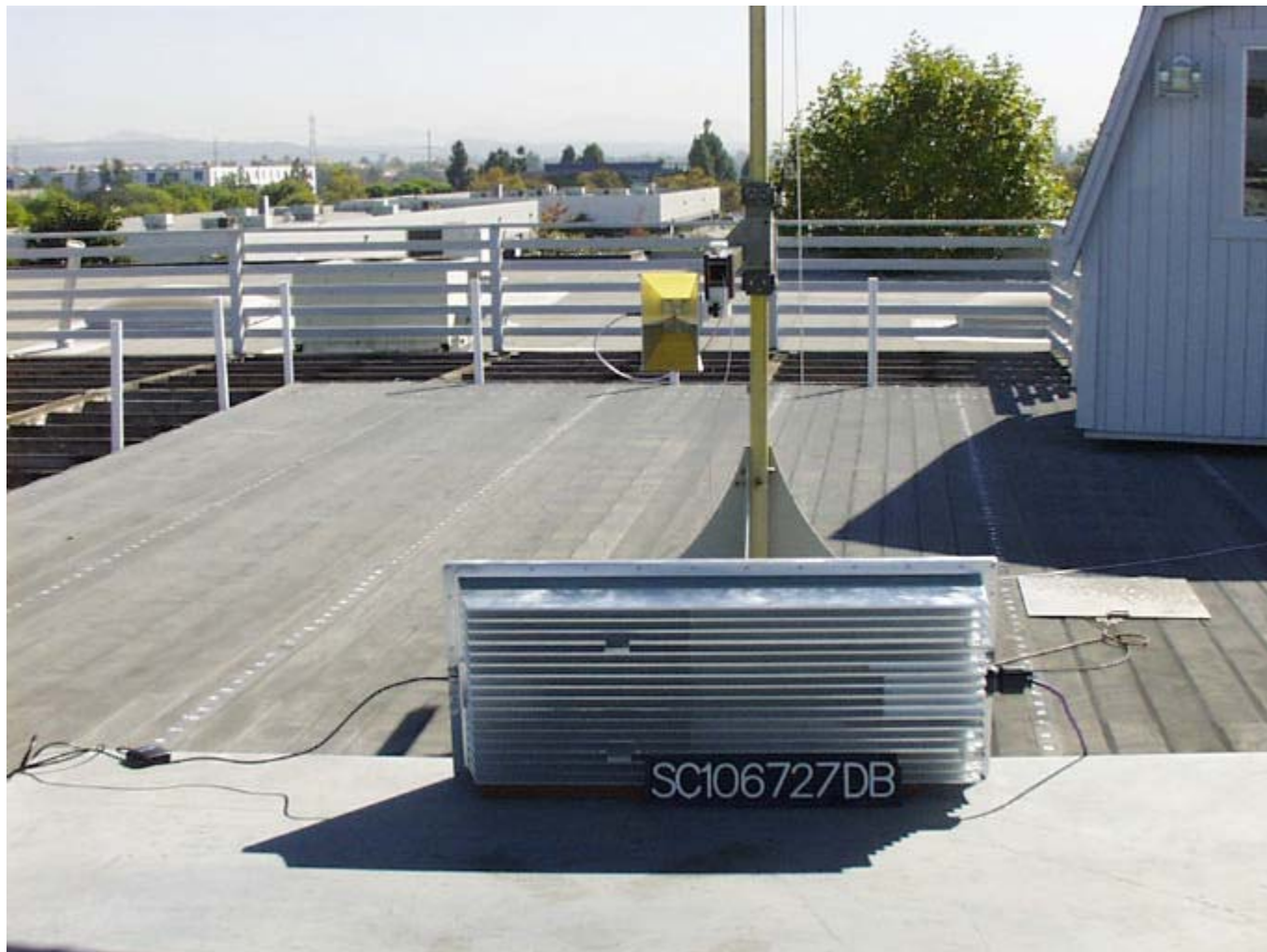
Photograph of Test Setup: Radiated Emission in Restricted Bands and Radiated Emissions
