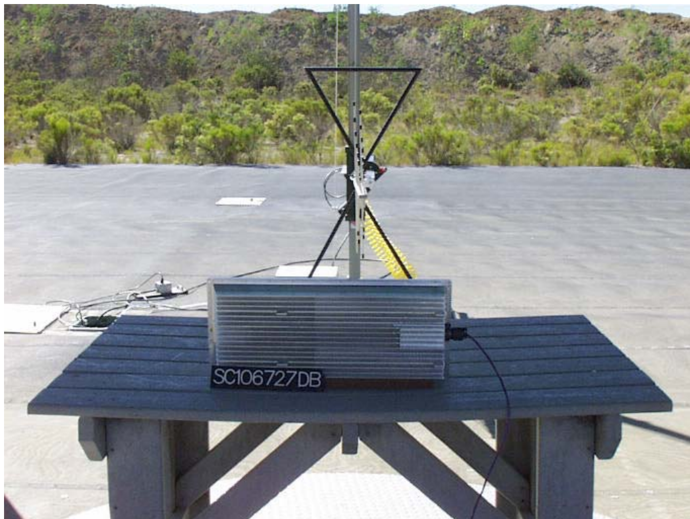
Photograph of Test Setup: Radiated Emissions
