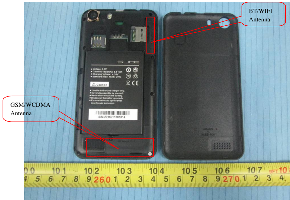
EUT –Cover off View 1
