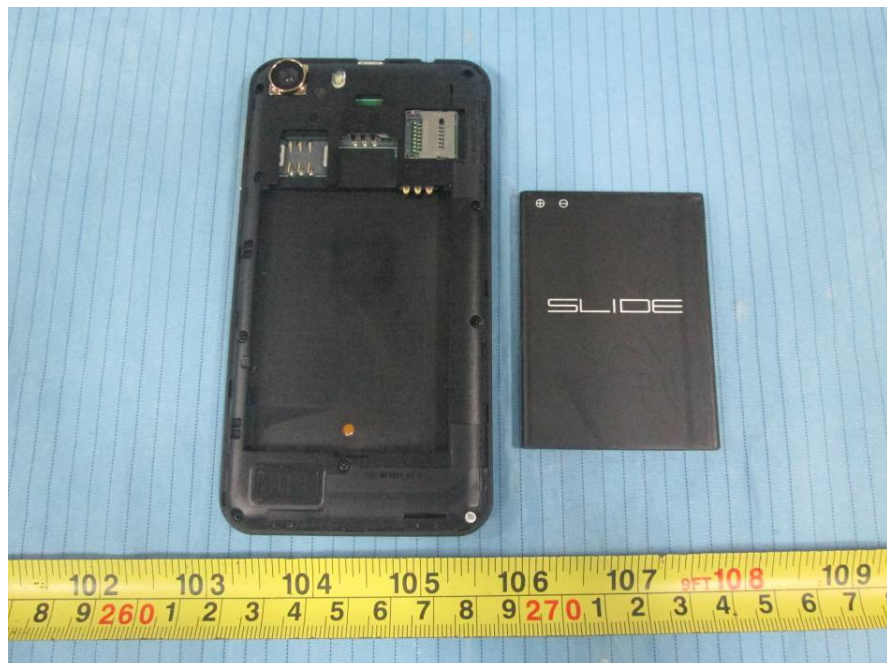
EUT –Cover off View 2
