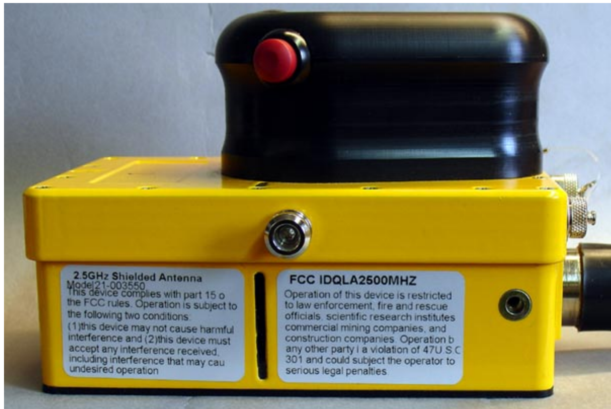
Figure 2. Placement of the FCC labels at the left side of the UWB-unit. Visible at all times.
